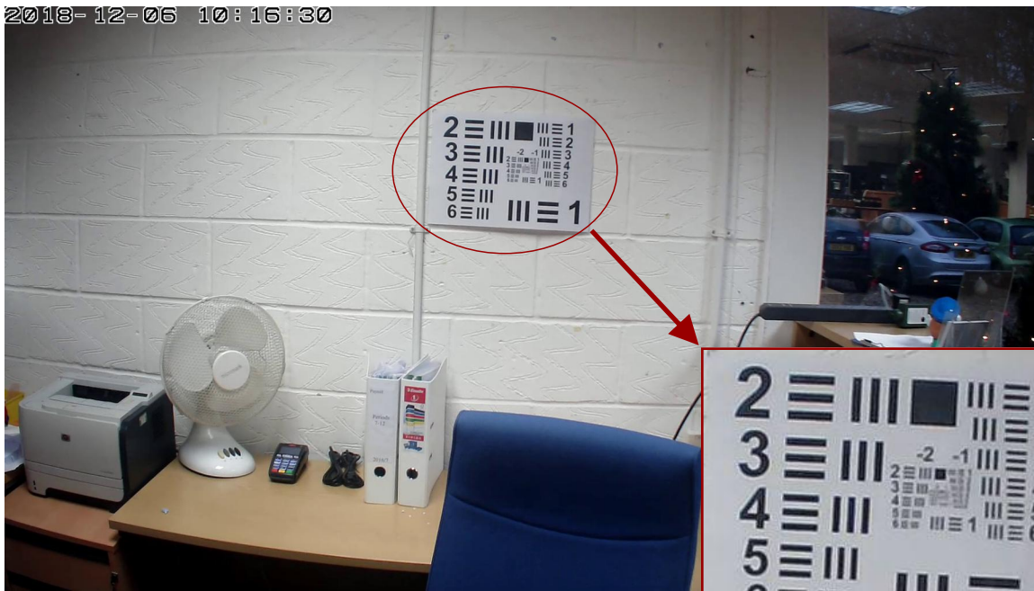
1080p (1920x1080 pixel) screen-shot with M12 4.3mm pinhole lens. Chart is 2.5 metres (8 ft) away.
