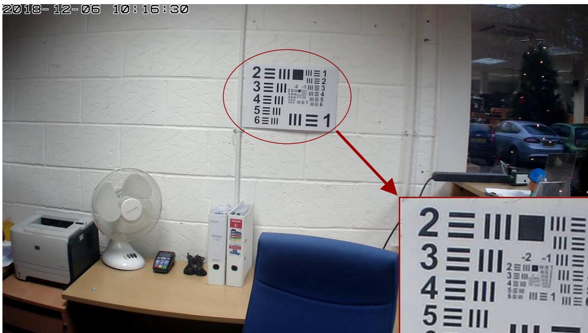
1080p (1920x1080 pixel) screen-shot with M12 4.3mm pinhole lens.
